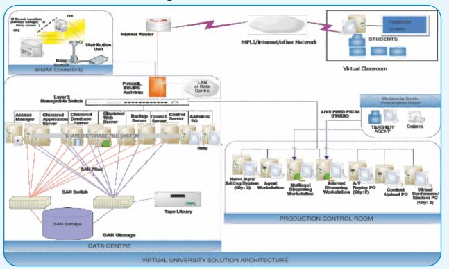
The Tele-Education solution is based on state of art technologies and uses diverse communication networks depending on the user requirements. The solution is modular, scalable, expandable and can grow with growth of user organization. The solution envisages data centres, studios & virtual class rooms for management of lectures, lecture content, lecture studios (teacher end), virtual class rooms(student end), programmes, courses, teachers etc.
